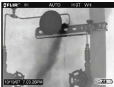
A leaking pressure gauge
