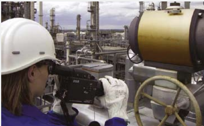
Examining potential leak paths
